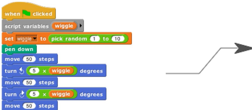
As in the **for** block, you can click on an orange oval in the **script variables** block without dragging to change its name. You can also make more than one temporary variable by clicking on the right arrow at the end of the block to add another variable oval:
